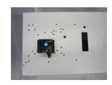
Mount the junction box according to the drilling pattern. Use screws M3.
