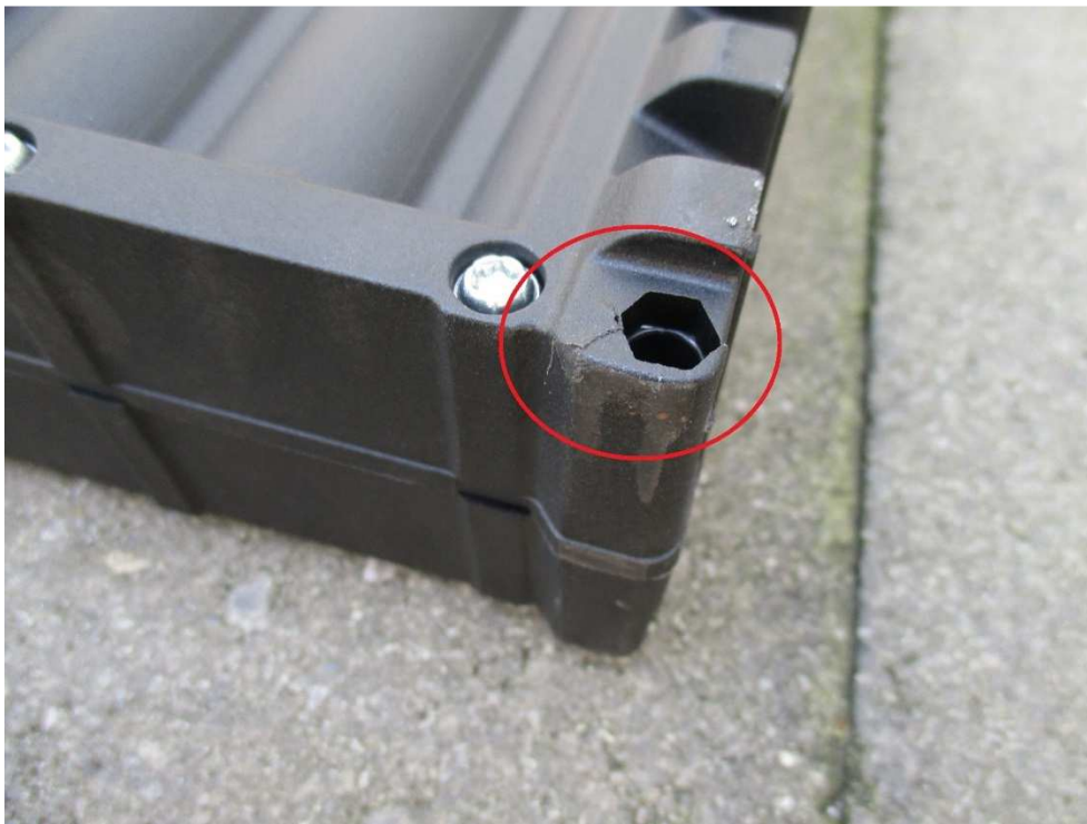
Picture 8 Crack in the enclosure after the test
