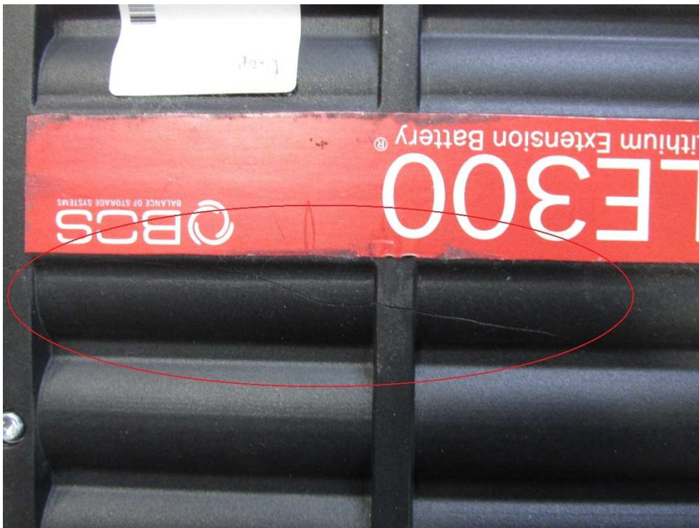
Picture 6 Crack in the enclosure after the test
