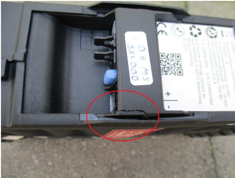
Picture 7 Crack in the enclosure after the test
