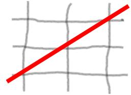
If you glue in serpentine water can escape. The distance of the turns should be about 8 to 12 cm.
