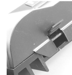
4.) Insert the sensor connector in the opening made in the casing so that the sensor cable can be run along the rear side of the regulator to the battery.
