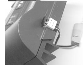
5.) The sensor should be laid so that it is as close as possible to the battery. It should be possible, for example, to screw the eyelet of the sensor directly to one of the two pole terminals. If necessary you can elongate the cable by yourself with a similar cable up to max. 5m.
